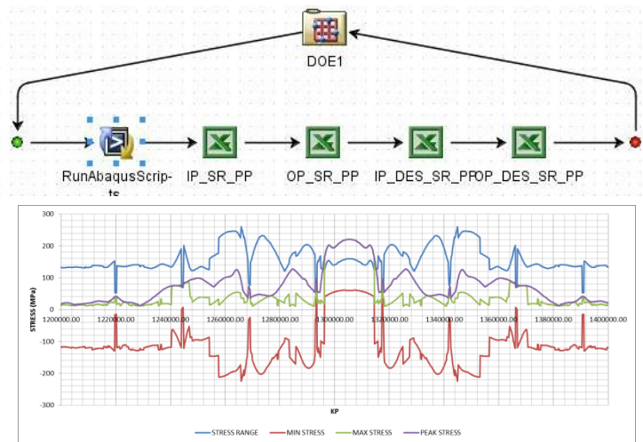
Figure 21. EOL stress and stress ranges calculation Isight process and typical graphical response in Excel components
