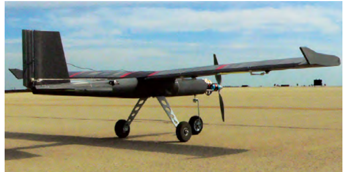
Shown prepped for test flight, this UAS by SelectTech Geospatial with all-FDM airframe was the first such craft to take off and land on its own power.
