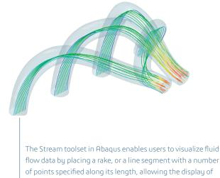
flow data by placing a rake, or a line segment with a number of points specified along its length, allowing the display of fluid flow in the model. An example application is a conjugate heat transfer analysis of an exhaust manifold.
