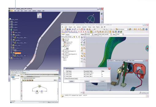
Perform seamless parameter updating for design iterations with bidirectional associativity in Abaqus.
