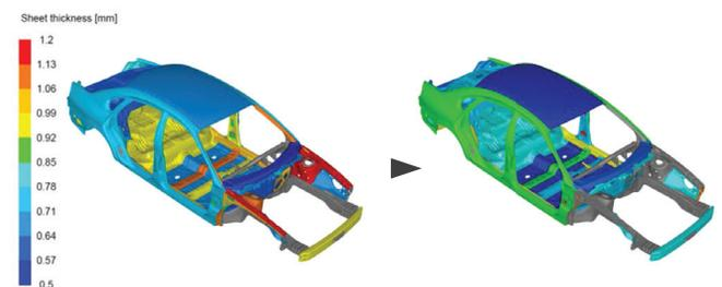
The optimal combination of weight, stiffness, and dynamic behavior using Tosca Structure.sizing resulted in a weight reduction of 15%—from initial 329 kg to 280 kg. While high stiffness requirements contribute to an increase in comfort, all other performance goals are met within a reduced development time.
